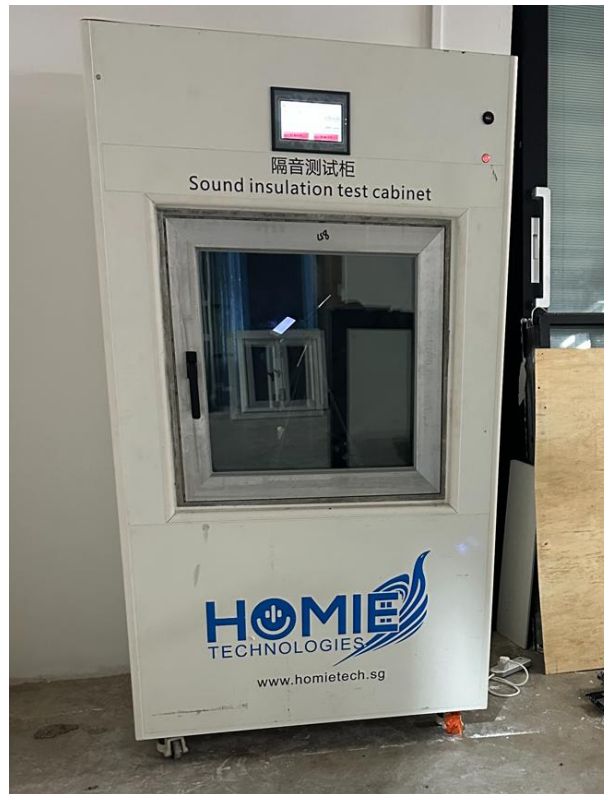
Figure 1.1: Sound insulation test cabinet.
