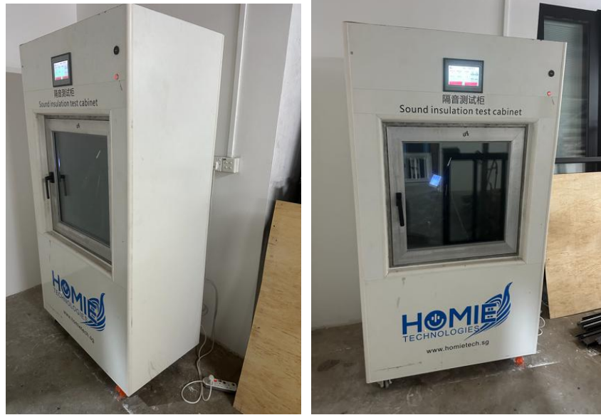
Figure 2.1: Test cabinet setup at site for the measurement
